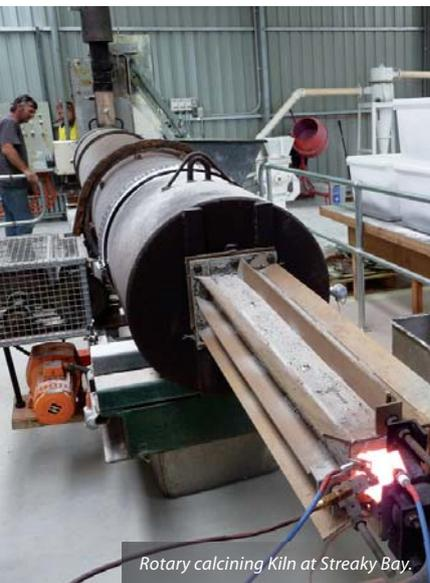
Rotary calcining Kiln at Streaky Bay.
