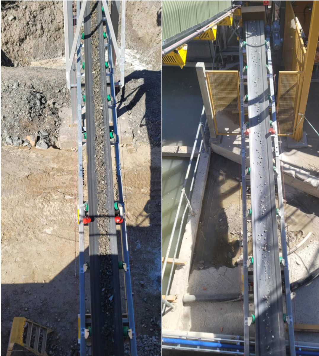
Figure 1 Output view from Ore Sorter. Greywacke waste rock on the conveyor on the left and quartz the host of the gold on the conveyor on the right.
