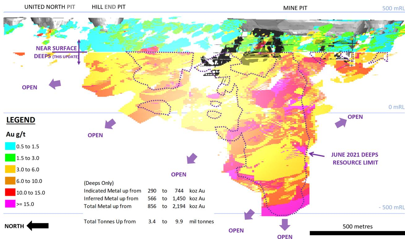
Figure 4 - Deeps Resource and Near Surface Resource Model Au grade distribution in area near pits, showing progression of Deeps Model from June 2021 (Deeps is below 300 mRL).
