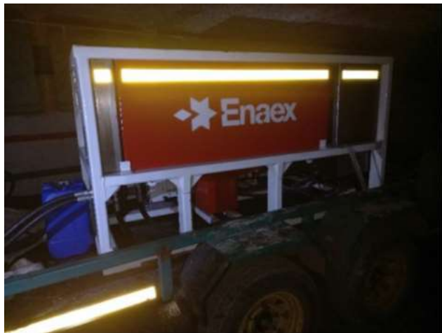
Figure 6 & 7- Bulk emulsion explosives charging unit
