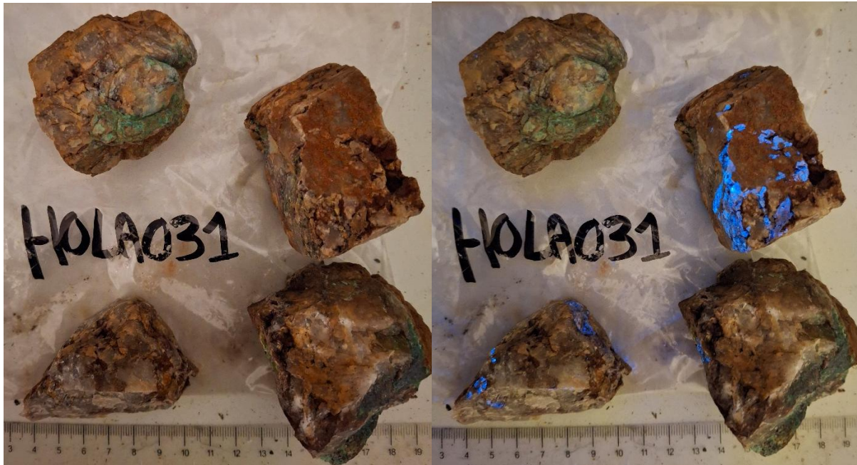
Figure 4: Examples of fluorescent blue scheelite mineralisation and green copper mineralisation from the Old Ghans Prospect (HOLA031) within the Hill of Leaders Project, NT. Left=normal light, Right=UV light
