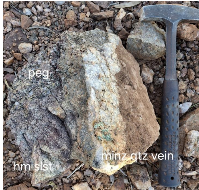
Figure 5: Example of mineralised (malachite-chalcocite-wolframite) vein from Old Ghans. The sample show granite (“peg”) intruding a hematitic siltstone and both are intruded by the mineralised quartz vein
