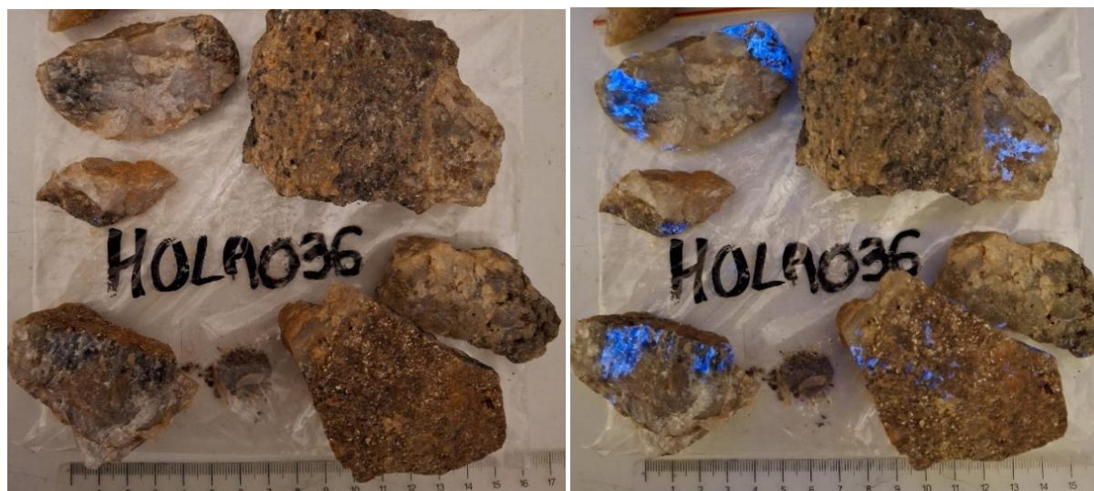
Figure 1: Examples of fluorescent scheelite mineralisation from the Doria Prospect (HOLA036) within the Hill of Leaders Project, NT. Left=normal light, Right=UV light
