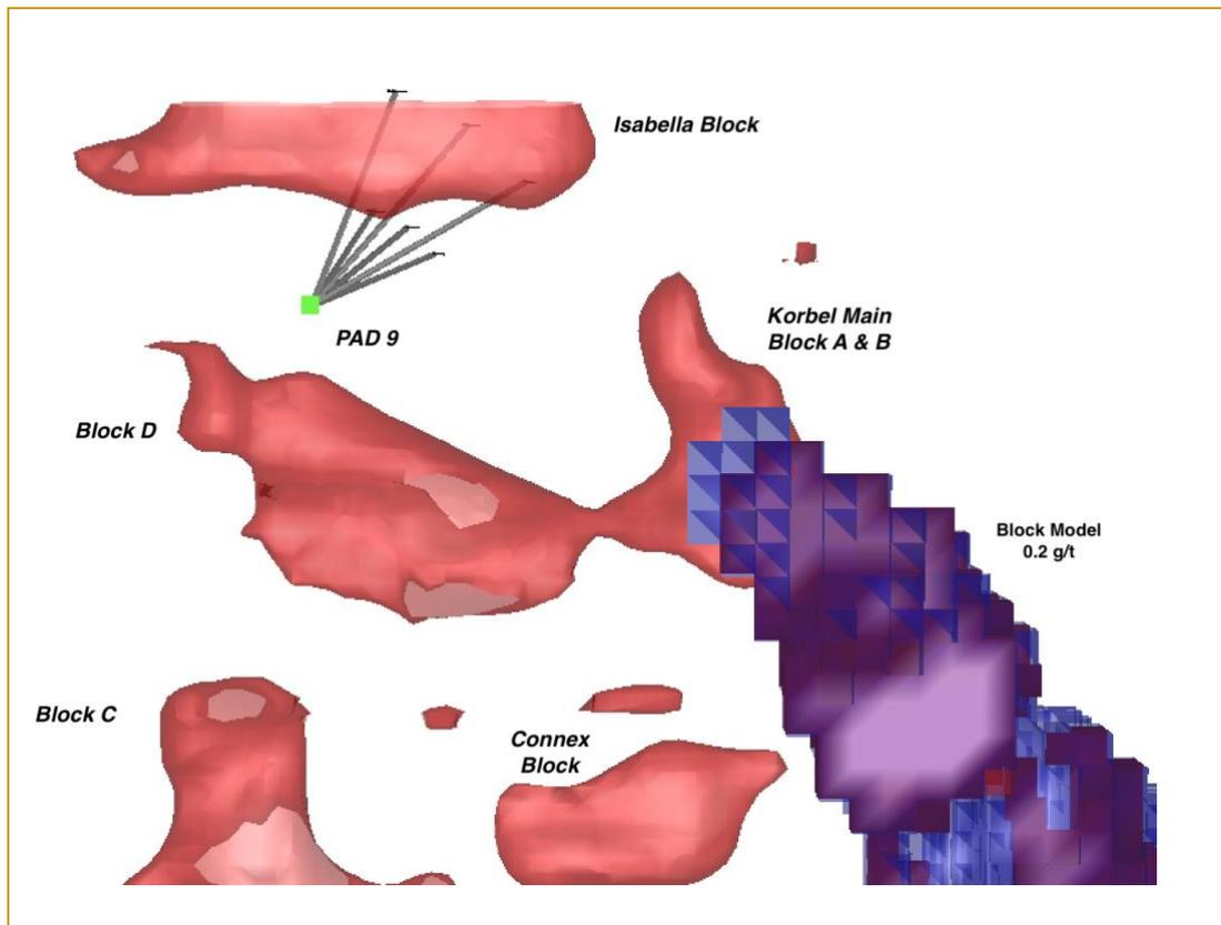
**Figure 2.** Isabella Drill hole layout with 3D IP Chargeability Anomalies (15 mV/V) and Block Model
