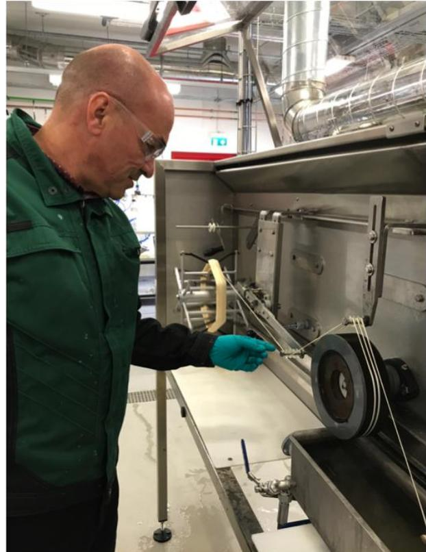
*Nullarbor fibre going through the spinning process using standard industrial equipment.*
