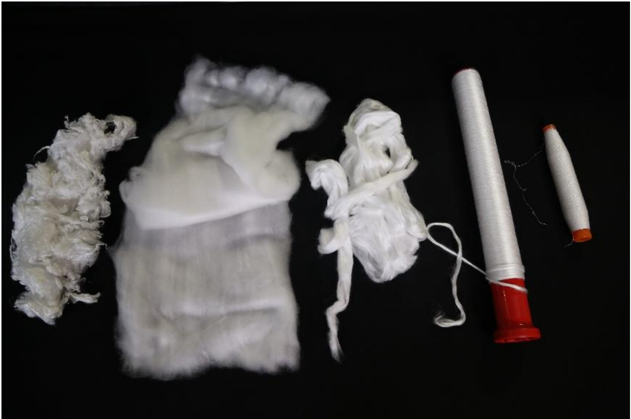
The Company's 100% Tree-Free Nullarbor™ Lyocell fibre at various stages in the process from fibre to yarn, being from left to right: Raw Fibre; Carded Fibre (Beard), Sliver (6x Carded Beards); Roving (1x Sliver); Ring Spun Yarn.
