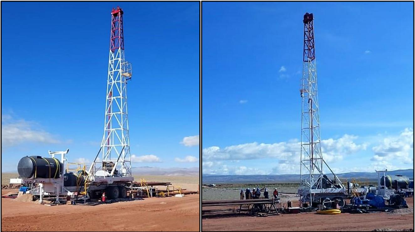
**Figure 2.** The rotary drill rig operating at the first drillhole at Lake’s Olaroz Project.
