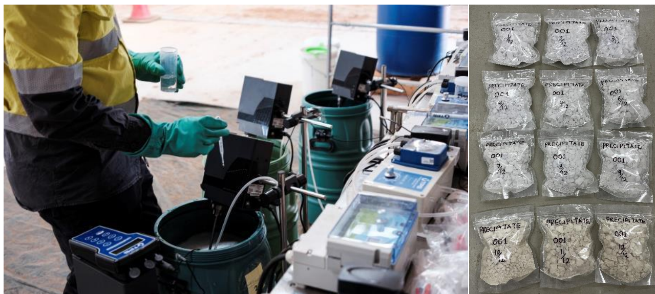
Figure 2: Demonstration plant precipitation circuit and inventory of MREC samples being dispatched to Australia for analysis.
