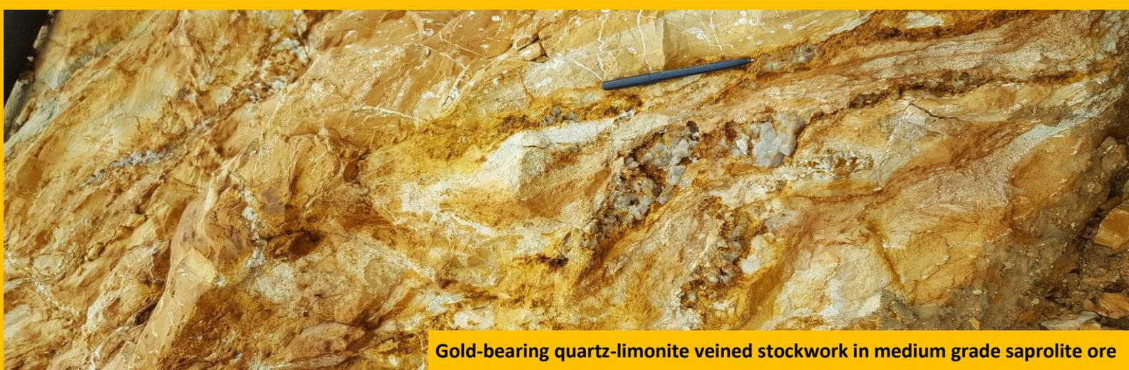
**Gold-bearing quartz-limonite veined stockwork in medium grade saprolite ore**
