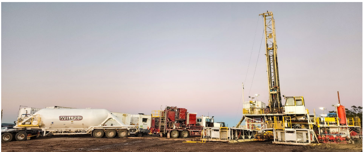
Picture 2: Cementing operations. Photo credits: Molly McEwin
