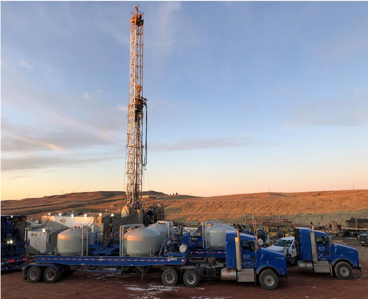
*CapStar #311 Rig on location performing surface cement job*
