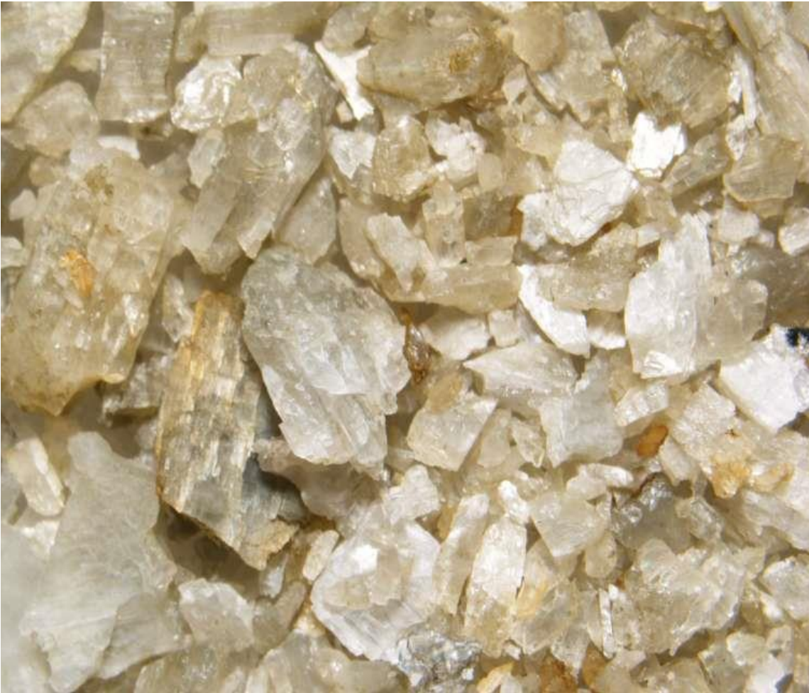
Figure 2. 8.10% Li 2 O Spodumene Concentrate from HLS Testwork on Grants.
