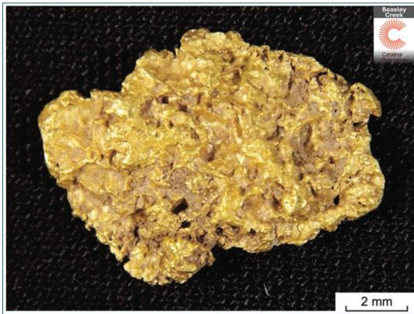
Figure 10. Gold nugget from Beasley Creek, with angular character, from GSWA, mineral report on sample 210968
