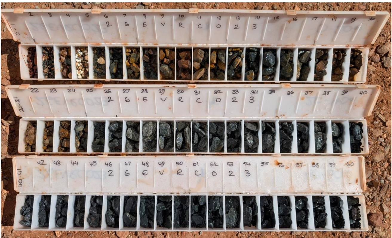
Figure 8. Representative RC rock chip samples from drill hole 26EVRC023 (0–60 m), Viper Prospect
