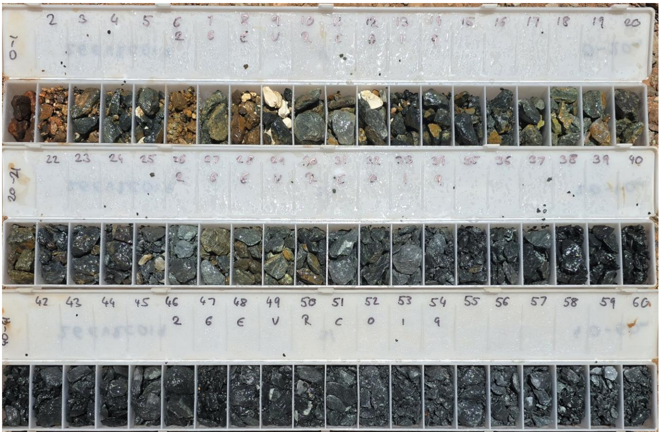
Figure 5. Representative RC rock chip samples from drill hole 26EVRC019 (0-60 m), Viper Prospect
