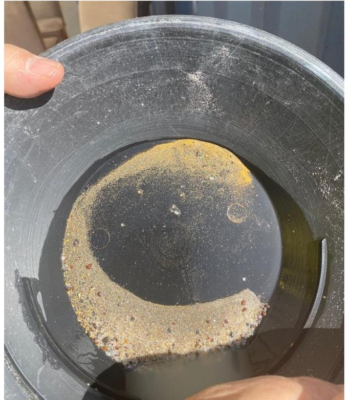
**Figure 3: Gold from Kat Gap ore in panning dish.**
