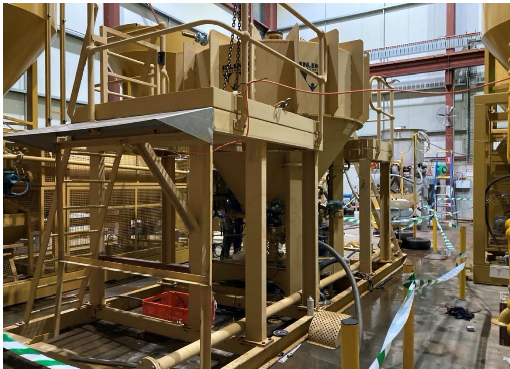
Figure 3: Classic's "IPJ" (Inline pressure Jig) Module during its refurbishment at Gekko, Ballarat, Victoria.
