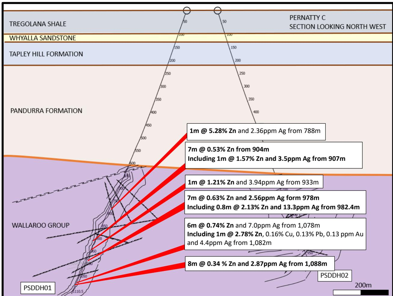
Figure 2: Cross Section looking north-west of PSDDH01 and PSDDH02 from surface with cover stratigraphy and folded and faulted basement Wallaroo Group metasediments
