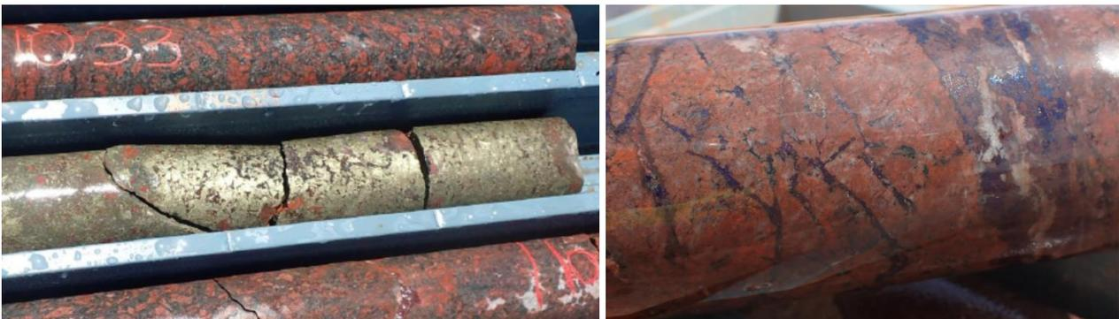
Figure 2: Pervasive chalcopyrite + pyrite mineralisation in altered, hematite-rich granite (left hand photograph) and bornite + chalcopyrite stringers in hematite-rich, altered granite (right hand photograph)
