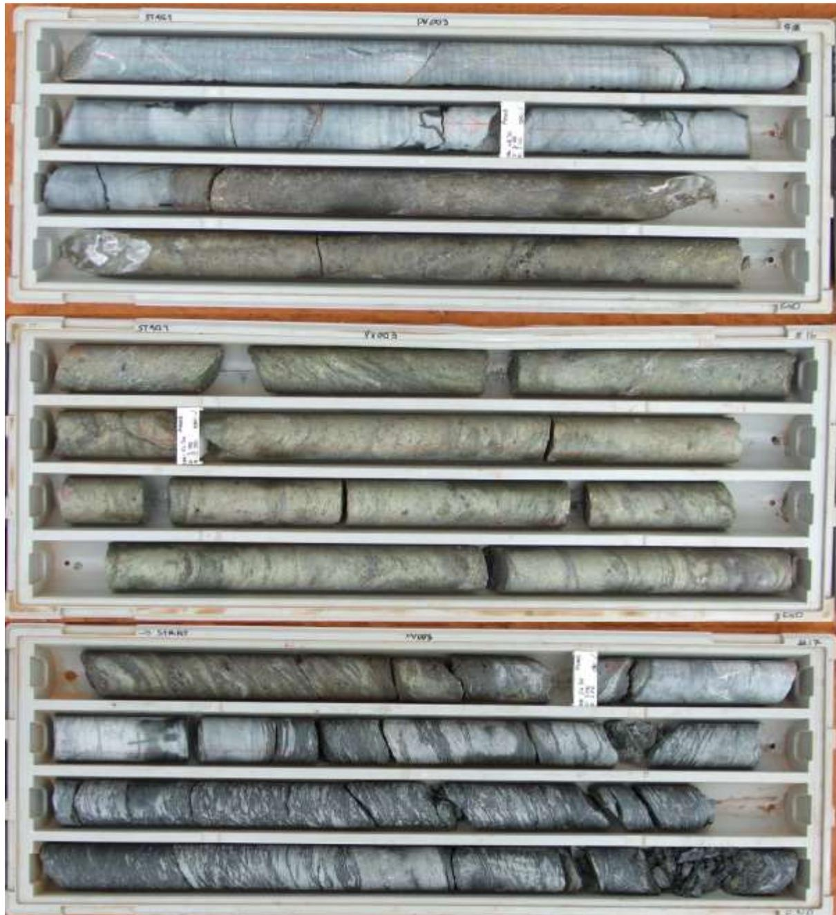
**Figure 1: Diamond core trays containing VMS mineralisation from the Schwabe Prospect (tray numbers 15-17 including 48.8m to 54.3m depth in hole 20PVDD003)**
