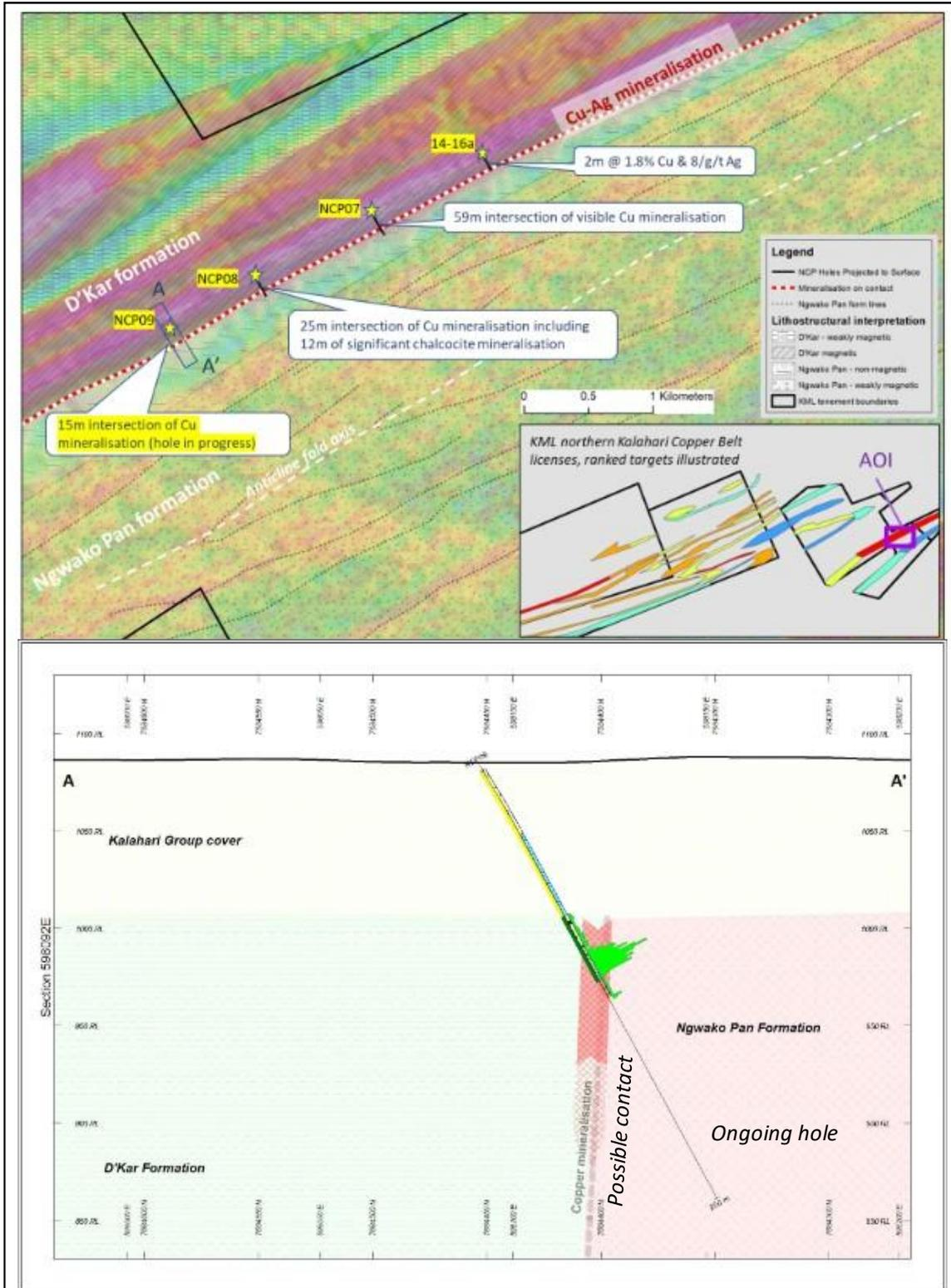
Figure 2. Plan view (above) illustrating drill positions on airborne magnetic data. Section (below) through NCP09 illustrating mineralisation (green plot) related to the D'Kar / Ngwako Pan formation contact.
