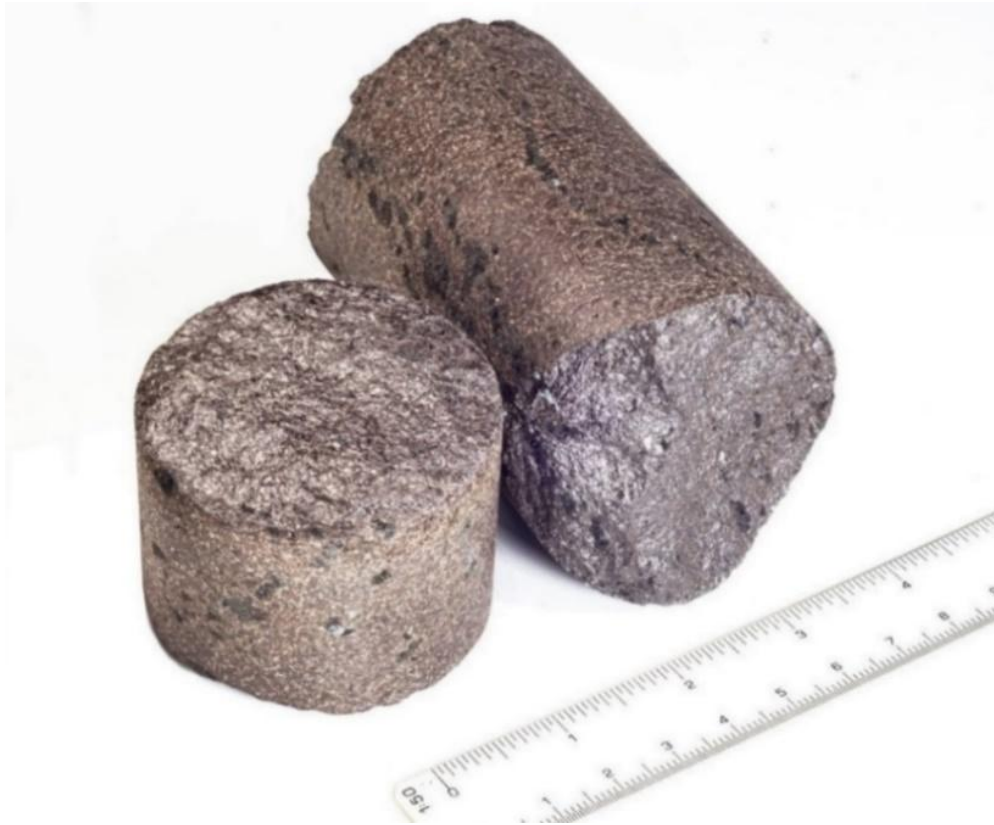
Figure 5: Ultra-high-grade core sections with chevkinite mineralisation (brown) and accessory apatite-britholite (pale flecks)
