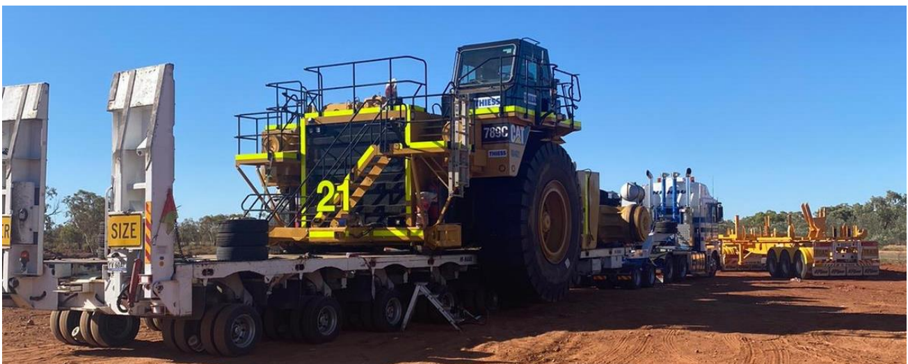
Figure 1. Thiess truck arriving at Anthill mine for assembly.
