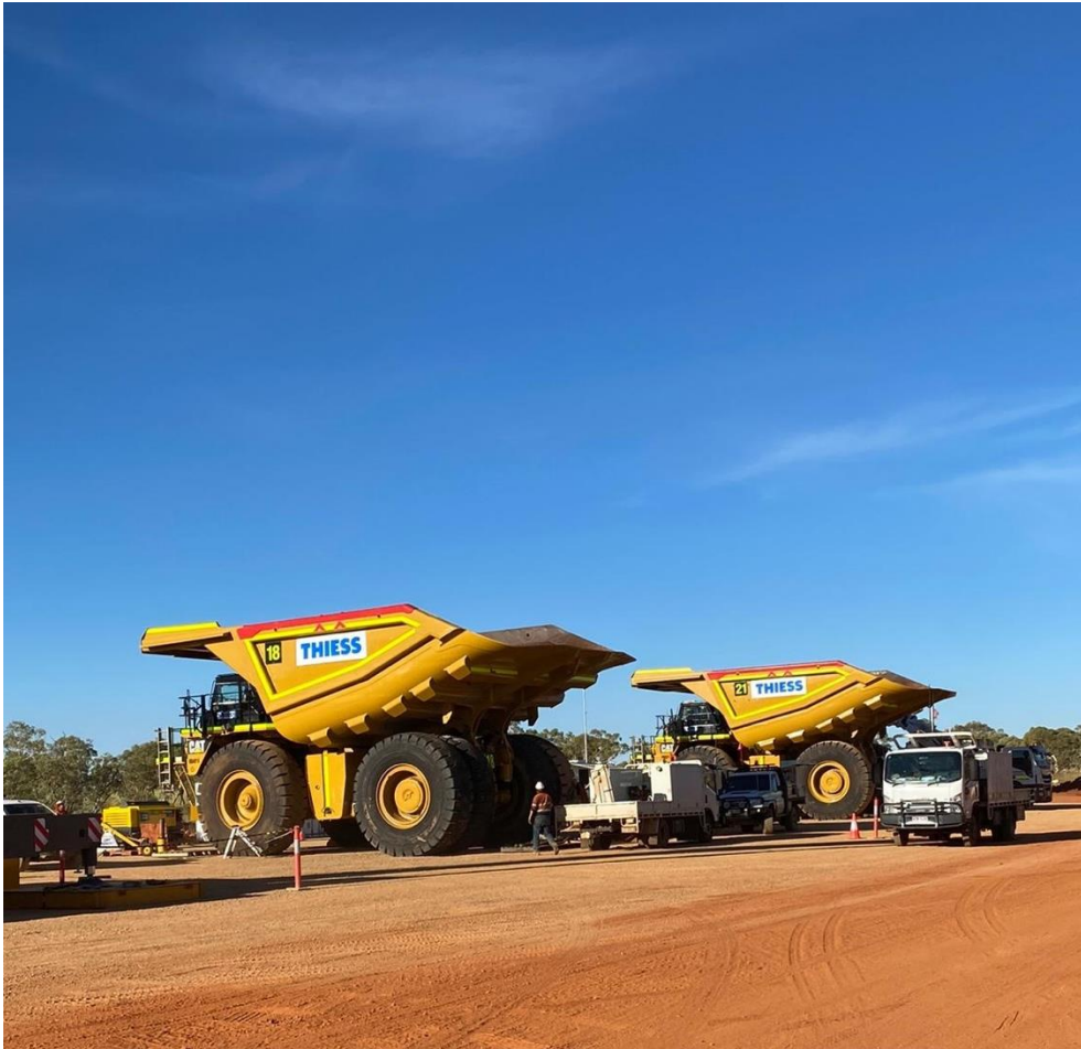
Figure 3. Cat789 trucks being assembled at Anthill.
