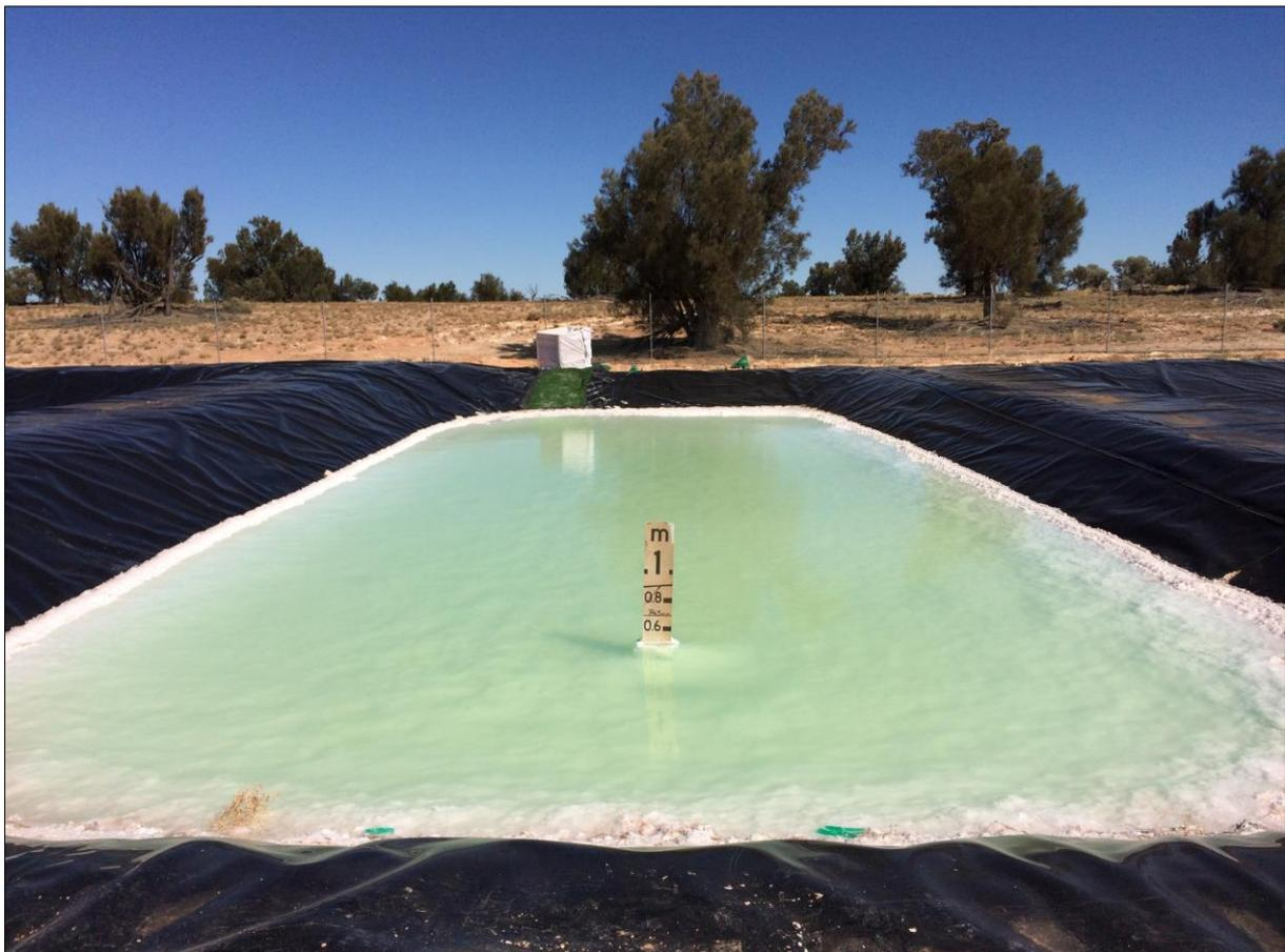
**Figure 1:** H1 containing saturated brine and precipitated K and SO<sub>4</sub> bearing salts prior to second brine transfer into H2
