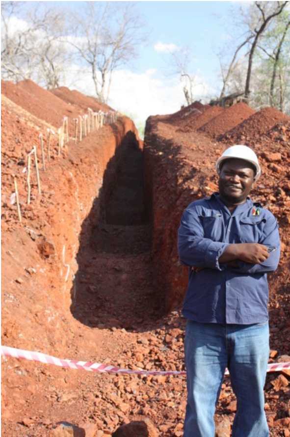
Plate 2: Senior project geologist, Norman Gwaza, poses at the foot of the southern Tenge trench. Stakes indicate sample intervals
