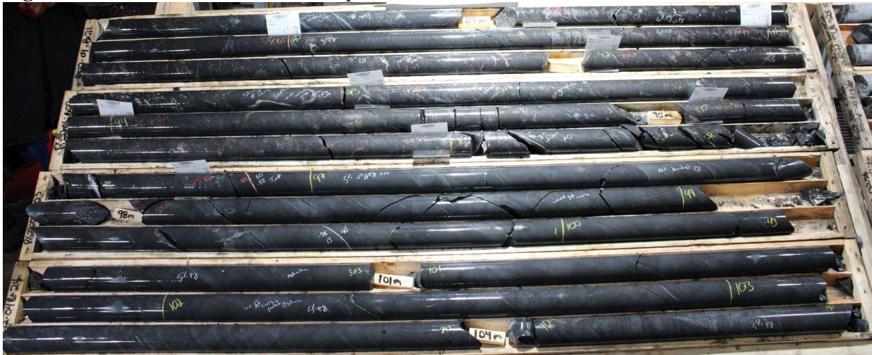
Figure 2: Core Photo - RS-22-04 Graphitic Interval - 88.3 to 96.9 m
