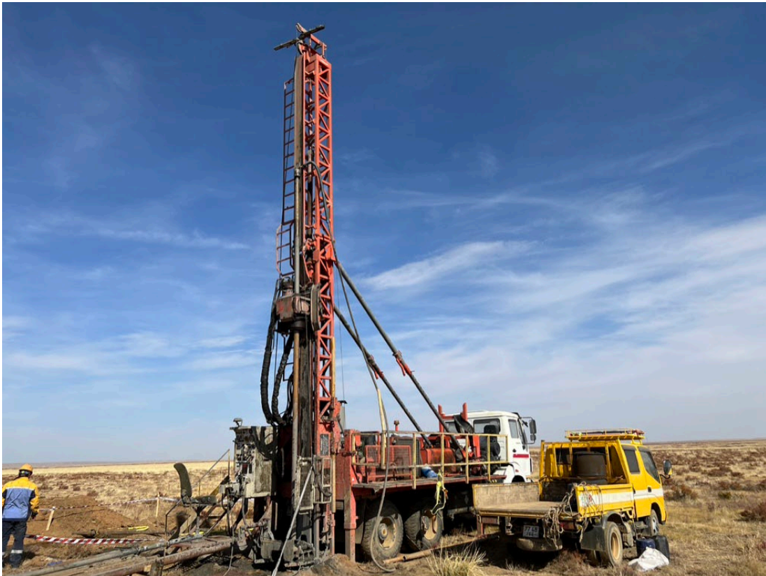
Figure 4. Diamond core drilling at UNDH-02.
