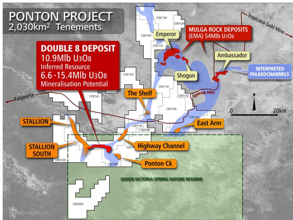
In November 2009 GPX Surveys flew a combined helicopter electromagnetic ("EM") and airborne magnetic survey over Manhattan's tenements in the Double 8, Stallion and Stallion South area. The EM survey results, along with earlier Manhattan EM surveys to the north, have clearly defined conductive palaeochannels prospective for sand hosted uranium mineralisation extending for over 130km within Manhattan's Ponton tenements.
