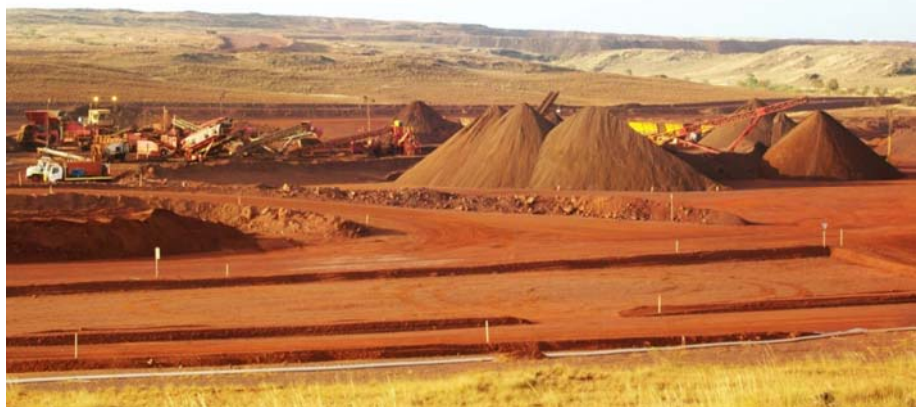
Figure 1: Upgraded DSO crush and screen plant at Pardoo capable of 2.4Mtpa
