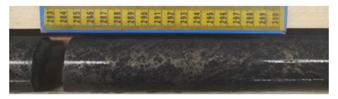
Drill hole KF21016 was designed as a 100 m step-out to the south of hole KF21013-015 to test the continuity of sulphide mineralization along strike. The hole did not intersect a significant mineralized horizon, however borehole electromagnetics "BHEM" indicate that the strongest part of the conductor is located off-hole to the northwest.
