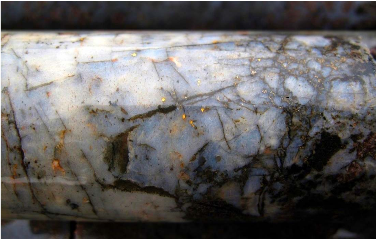
Visible gold in drill core from Challenger West drilling in Diamond Drill Hole 11CUD0783
