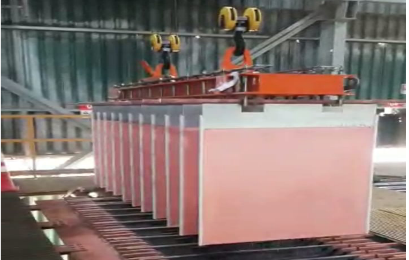
Figure 3 | Copper cathode being harvested at the Sierra Atacama SX-EW plant
