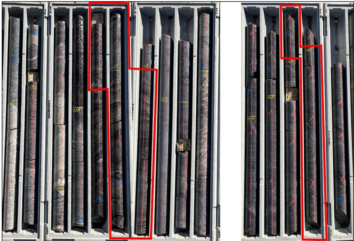
Figure 2. Sulphide rich zones in BDCDD2503 at 170.5m-172.5m downhole and 194.9m-195.9m downhole (for results refer appendix 1)
