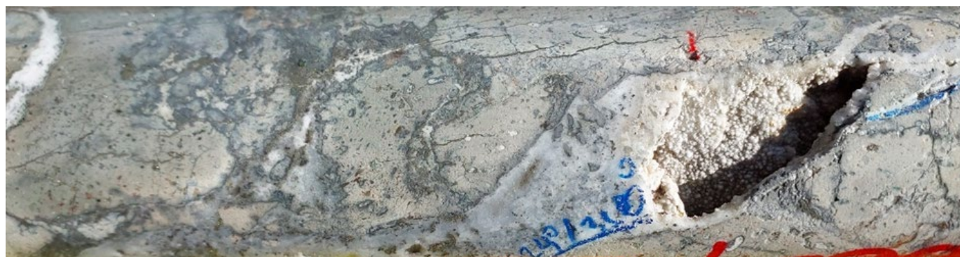
25VDD002_198.25-198.52m. From Sample No 386654, 198.25-198.67m (0.42m) 0.57 g/t Au, 5.28 g/t Ag. Mineralised chalcedonic vein breccias cemented by chalcedonic quartz with colloform and crustiform epithermal vein textures and abundant blebby pyrite, sphalerite and dark grey sulphide. 5% pyrite-sulphide. Within strongly silica-clay-altered basalt. Open spaces with druse silica.
