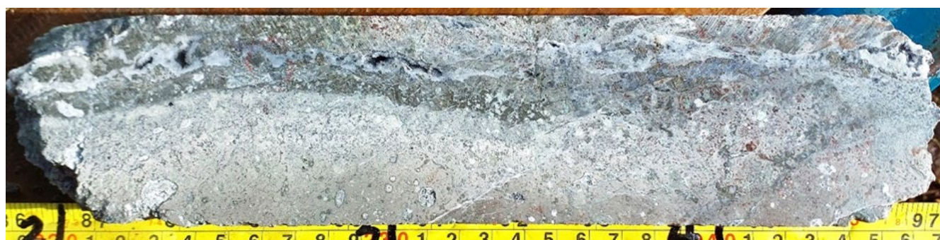
25VDD002_199.58-199.83m. From Sample No. 386656, 199.32-199.9m (0.58m), 26.4 g/t Au, 39.70 g/t Ag. Colloform banded and crustiform chalcedonic silica veins. Open spaces with druse quartz. Blebby and fine pyrite, sphalerite and galena-tennantite-tetrahedrite. The host lithology is a vesicular basalt and silica-clay-altered. Disseminated and blebby pyrite halo to the veins.
