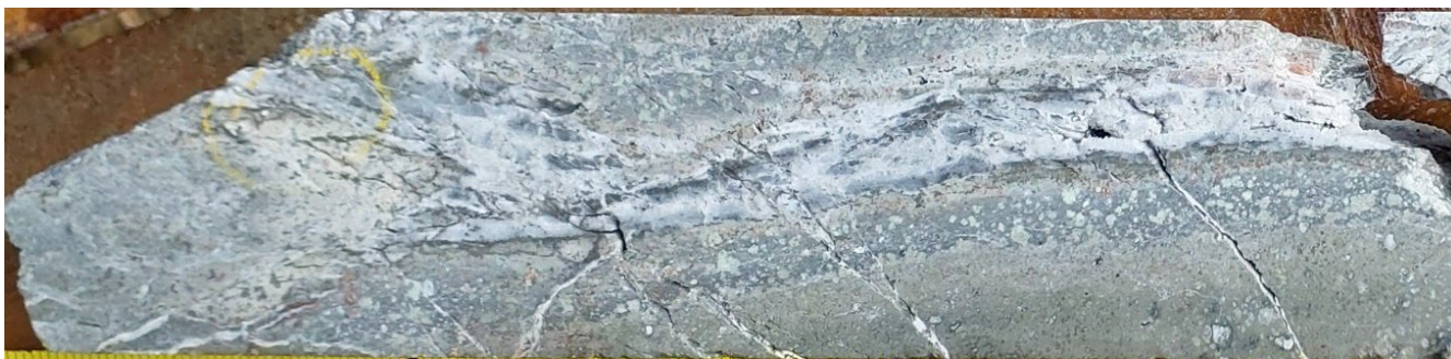
25VDD002_195.76-196.15m. From Sample No. 386651, 195.76-196.56m (0.8m) 11.4 g/t Au, 6.52 g/t Ag. Mineralised chalcedonic vein within strong clay-altered basalt. Colloform and crustiform epithermal vein textures, open spaces with druse quartz. Blebby and disseminated pyrite, sphalerite and grey sulphide.
