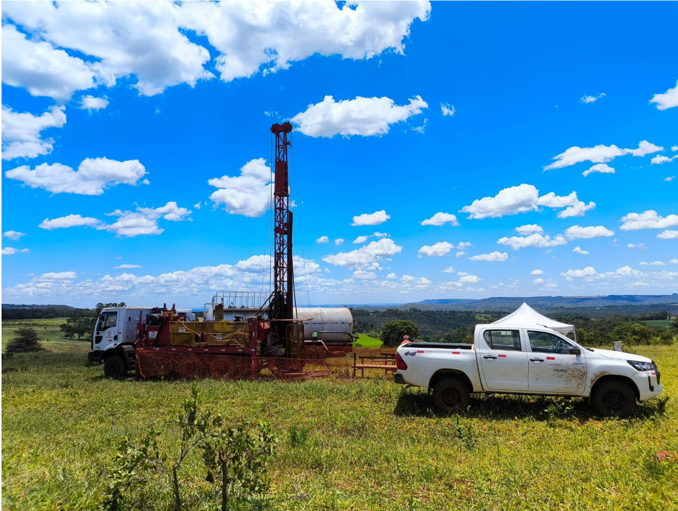
Figure 4: Active diamond drilling at the Olegario prospect, supporting mineralisation definition for the upcoming Maiden Mineral Resource Estimate.
