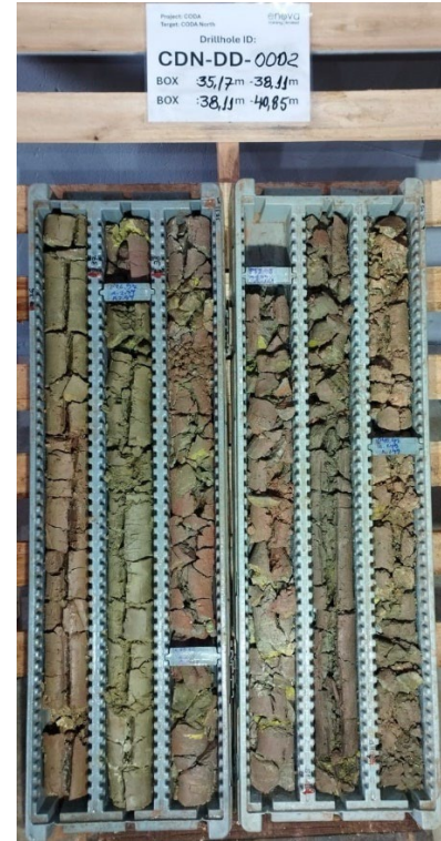
Figure 4: CDN-DD-0002 drill core which has been reported as having 14 m intercept @19.2% TiO 2
