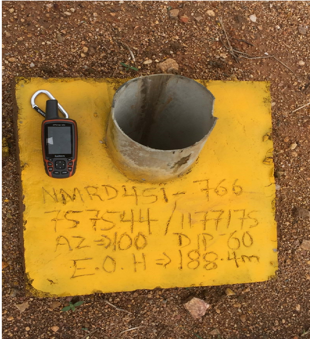
Figure 3.2.1_1 Example of a cemented diamond drill collar (NMRD451-766)
