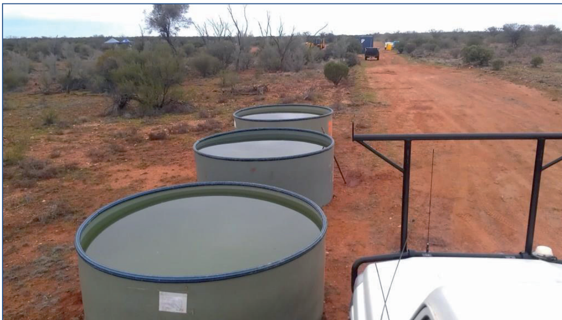
Figure 8. Evaporation tanks with 12,000 litres of brine at the start of the trial.
