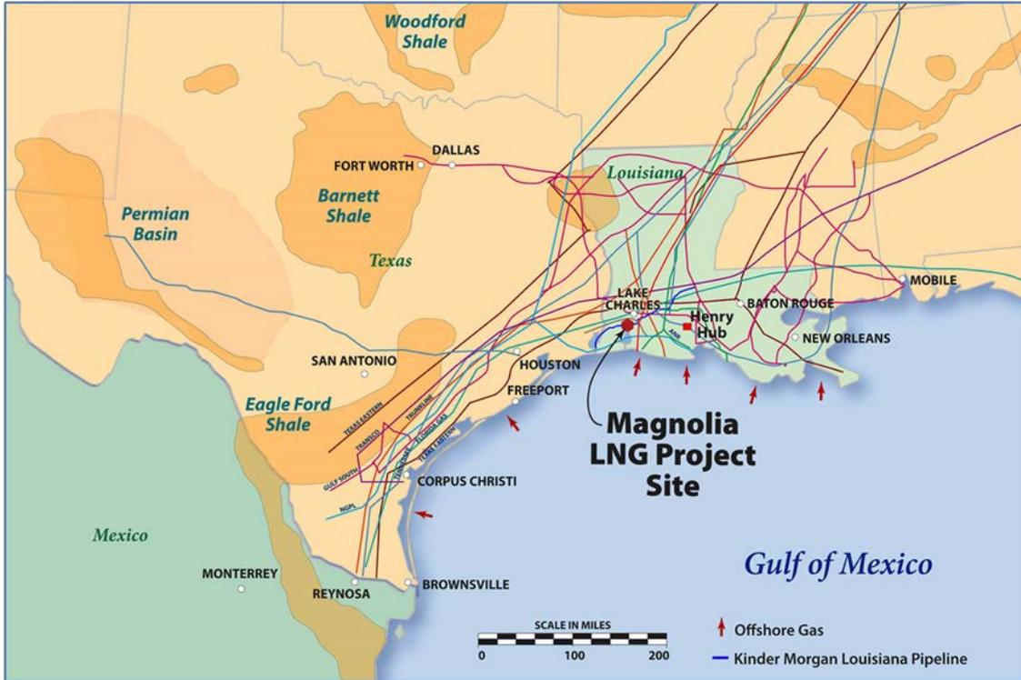
Map showing location of nearby unconventional Gas Shale Plays and connecting gas transmission pipelines (including KMLP) to the Magnolia LNG Project site
