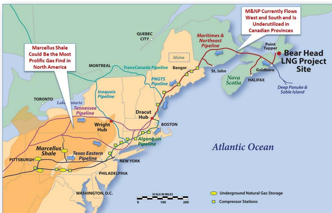
Location of the Marcellus Shale Play and natural gas transmission pipelines relative to the Bear Head LNG Project site
