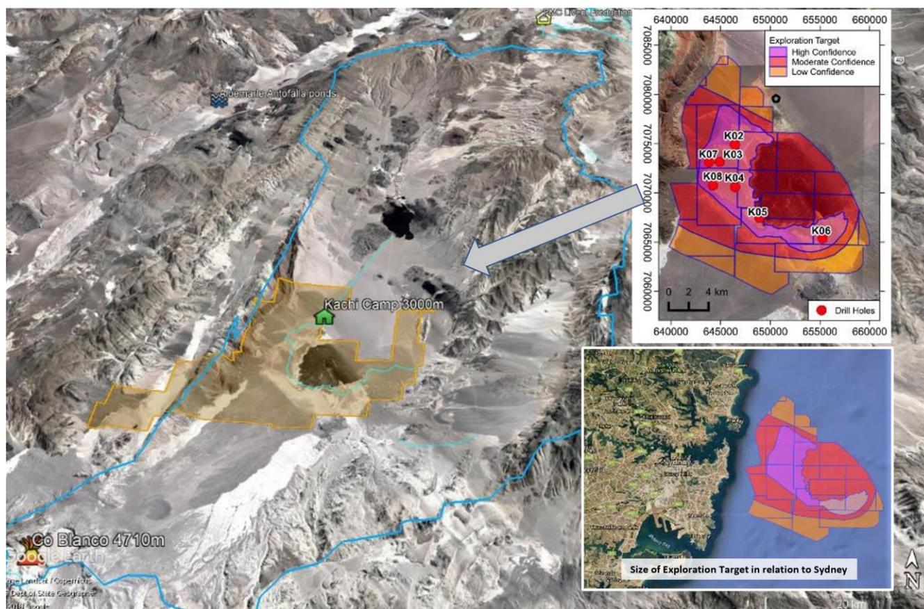
**Figure 4. Kachi Lithium Project showing mining lease boundaries (yellow) at the lowest point of a large drainage basin of 6800km<sup>2</sup> (blue line) with insets showing the Exploration Target of 8-17Mt LCE and the same target in relation to the Sydney basin.**
