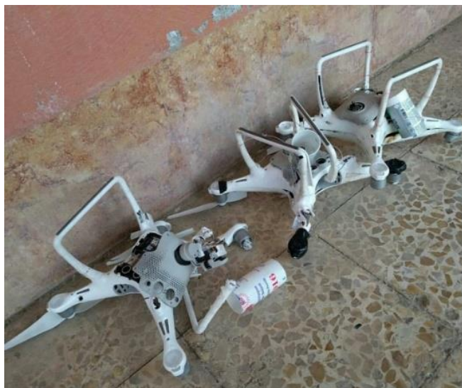
Image: Basic plastic tubes positioned underneath quadcopters appear right size for 40mm grenades 5
