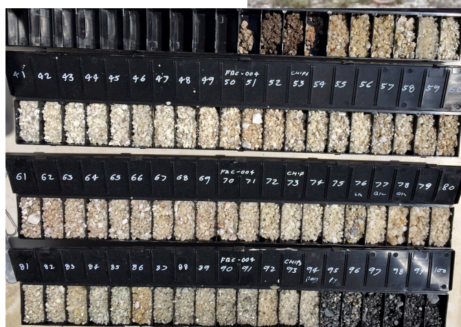
Figure 3 Drill cuttings from drilling program showing substantial pegmatite.
