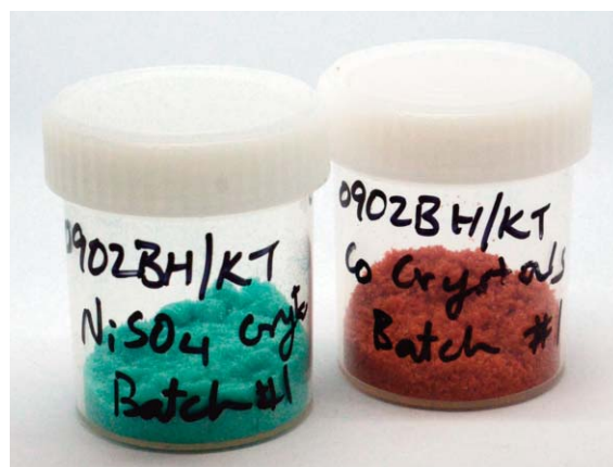
(above left) beaker nickel sulphate crystals, (above right) beaker cobalt sulphate crystals – laboratory testing of Goongarrie pilot plant output.
