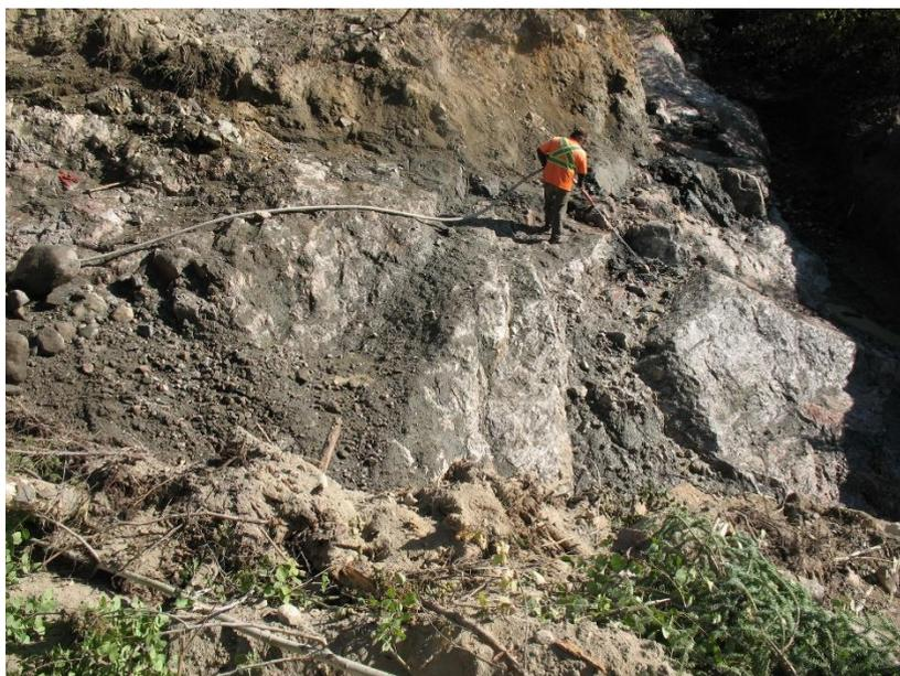
**Figure 4.** Worker washing down the newly excavated pegmatite structure located south of the North Aubry prospect to enable the geological team to review and identify the various lithium mineralisation zones.
