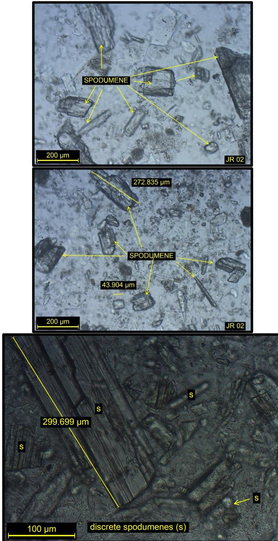
Figure 11. Images of coarse spodumene partials from thin section sample M221 JR002 -500
