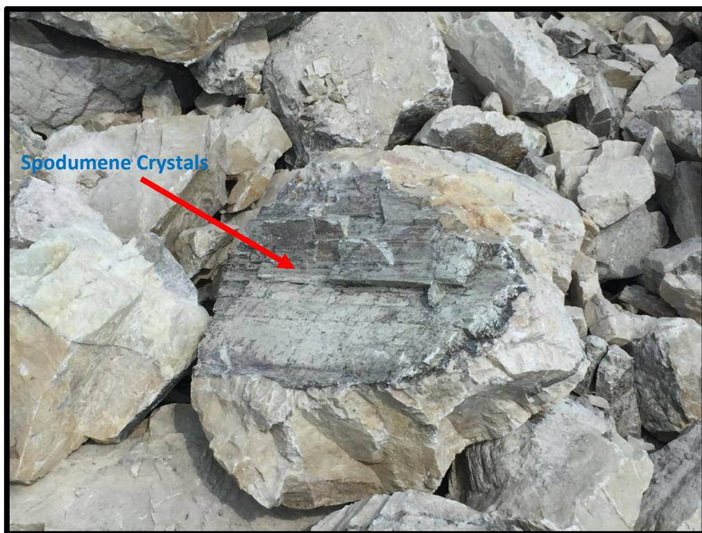
**Figure 9.** Bulk sample of Spodumene bearing pegmatite obtained from the North Aubry prospect. Highlighted in the image are the large high quality Spodumene crystals.
