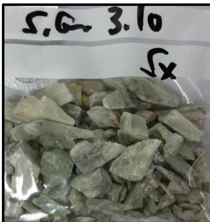
**Figure 13.** Sample of coarse lithium concentrate (Spodumene) created with DMS at the specific gravity of 3.10.
