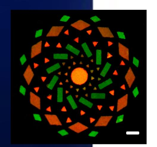
Microcode 'lights up' in multiple colours when excited via source of light (smartphone camera flash)
