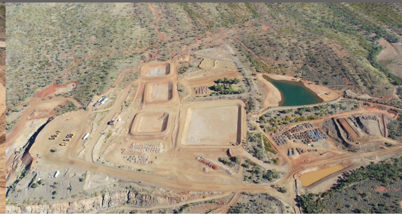
Above: GAM Crushing Circuit Below: Mt Freda Complex – showing VATs, storage ponds and stockpile areas
