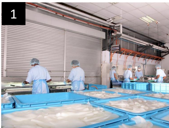
1 Fermentation with acetobacter xylinum to produce MC
